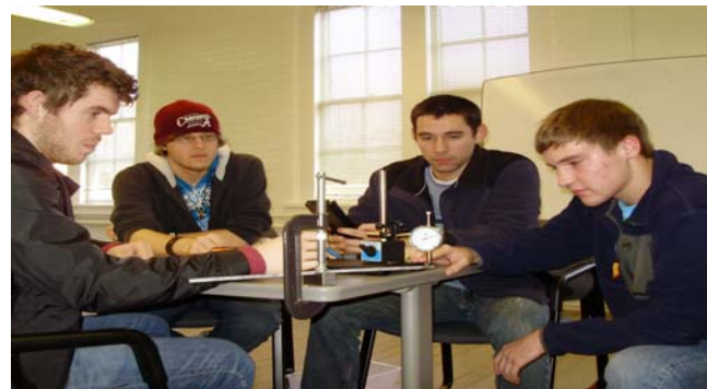
Students measuring the deflection of the cantilever beam under load with a dial gage.
