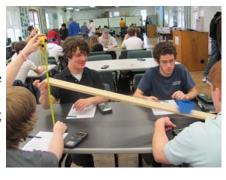
electrical box and a piece of wood. They measure both the static and kinetic coefficient of friction using an inclined plane. Mass can be easily added to the box to see the effect of that on the coefficient of friction. Based on these measurements they predict how far the box will slide on a level surface, and make
