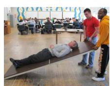
measurements to confirm their calculations. Finally, we use a large inclined plane to measure the coefficient of friction of a person. Dr. Bennett's coefficient of friction is 0.32.
